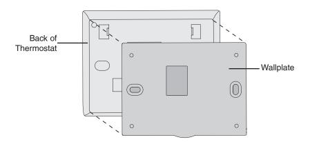
Drill 3/16" holes for drywall. Drill 7/32" holes for plaster.
